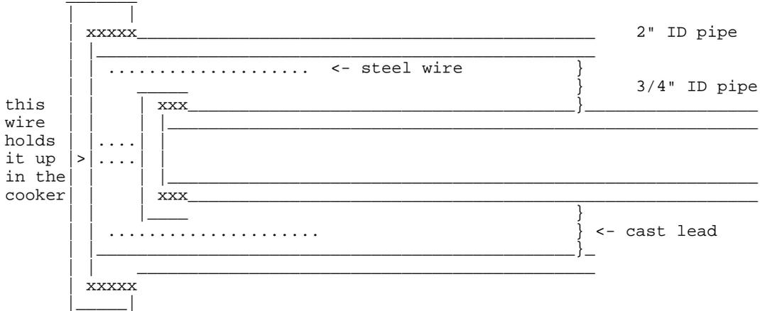
We dug into the side of a sand pile and built a chimney out of firebrick. Then we stood the assembled pipe and wire on end in the chimney, sitting on some bricks. We then had a blowtorch heating up the chimney, so that the pipe was red hot. Then we poured molten lead into the space between the pipes. If the caps aren't screwed on real tight, some of the lead will leak out. If that happens, turn off the blowtorch and the pipe will cool enough and the lead will stiffen and stop the leak.
