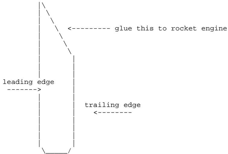
The leading edge and trailing edge should be sanded with sandpaper so that they are rounded. This will help make the rocket fly straight. A two inch long section of a plastic straw can be attached to the rocket to launch it from. A clothes hanger can be cut and made into a launch rod. The segment of a plastic straw should be glued to the rocket engine adjacent to one of the fins of the rocket. A front view of a completed rocket bomb is shown below.
