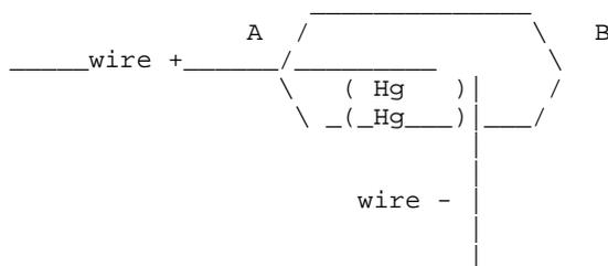
When the drop of mercury ("Hg" is mercury's atomic symbol) touches both contacts, current flows through the switch. If this particular switch was in its present position, A---B, current would be flowing, since the mercury can touch both contacts in the horizontal position.
