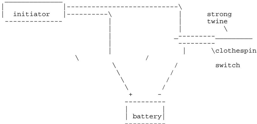
When the flat piece of wood is removed by pulling the string, the jaws of the clothespin will close, completing the circuit.
