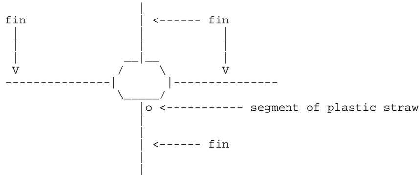
By cutting a coat hanger at the indicated arrows, and bending it, a launch rod can be made. After a fuse is inserted in the engine, the rocket is simply slid down the launch rod, which is put through the segment of plastic straw. The rocket should slide easily along a coathanger, such as the one illustrated on the following page:
