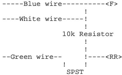
What this does in effect is keep the hookswitch / dial pulse switch (F to RR loop) open while holding the line high with the resistor. This gives the same voltage effect as if the fone was 'on-hook', while the 10k ohms holds the voltage right above the 'off hook' threshold (around 22 volts or so, as compared to 15-17 or normal off hook 48 volts for normal 'on-hook'), giving Test Set Version 2.
