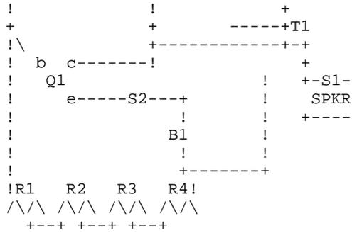
Now that you are probably thoroughly confused, let me explain a few minor details. The potentiometer area is rigged so that the left pole is connected to the center pole of the potentiometer next to it. The middle terminal of T1 is connected to the piece of wire that runs down to the end of the battery.
